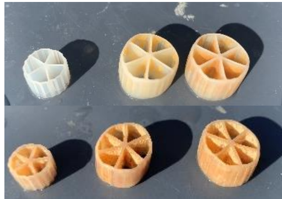
Figure 25 Biofilm Carriers aka 'Pasta Wheels' with bacterial growth.
