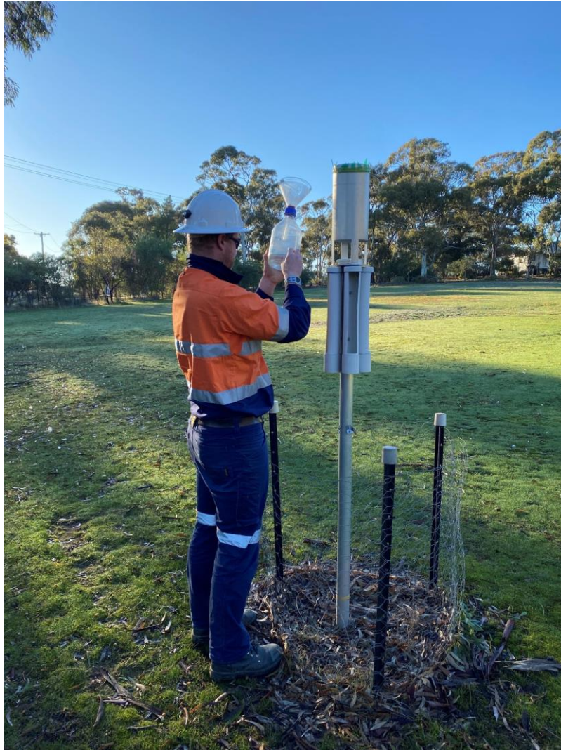
Figure 5 – Dust deposition gauge
